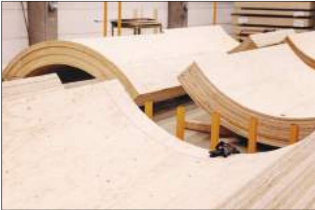
Test modules of wooden panels for wind turbine towers.
