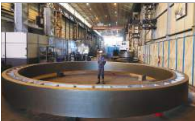
One of the dryer's trunnion rings, with an outer diameter of 9.06m, height of 0.66m, and weighs approximately 47 tonnes.
