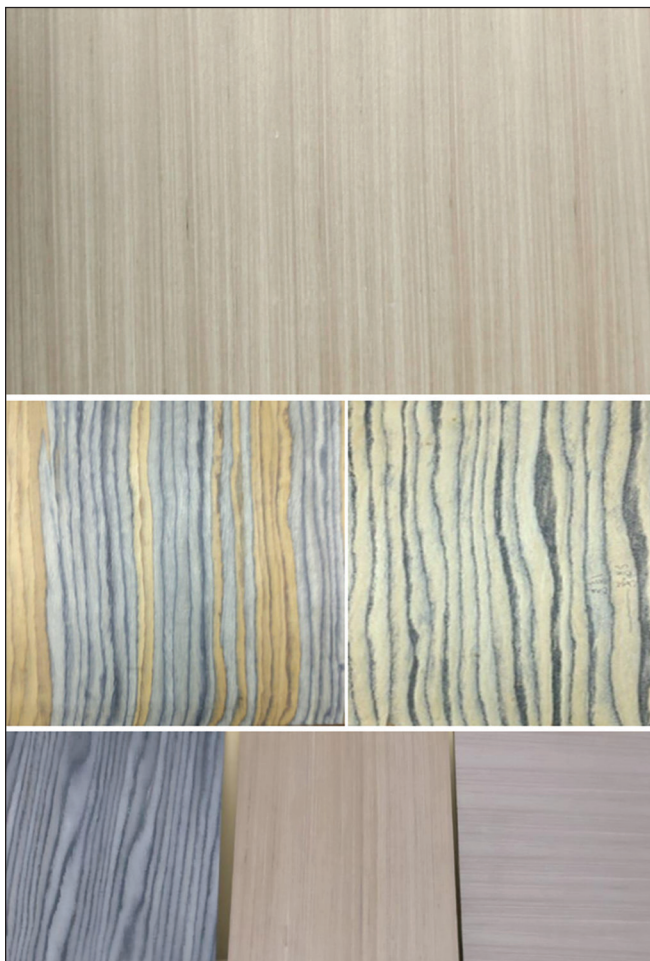
Figure 12: Different shades and designs of RECON face veneer made from poplar (Photo Dr. C. N. Pandey, Century Ply).
