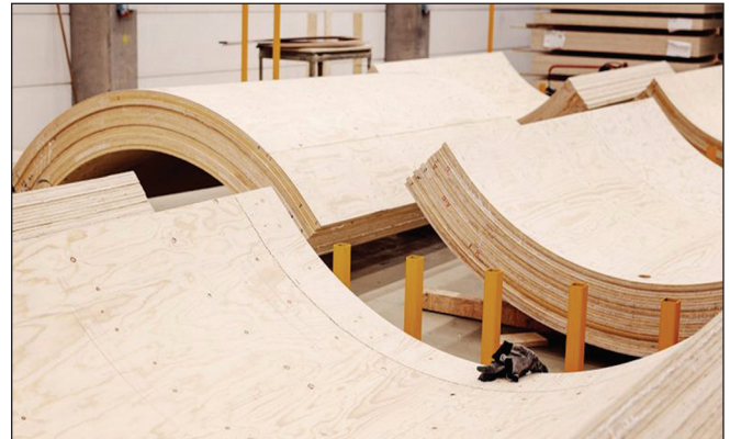
LVL modules of Modvion's wind turbine towers.
